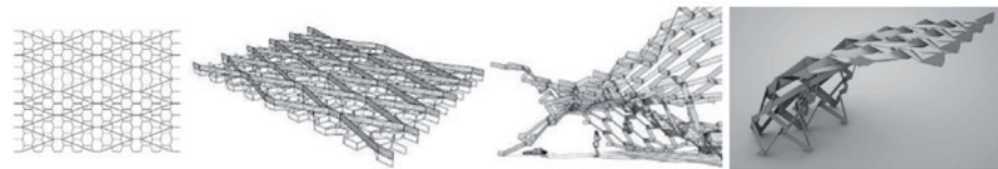
Figure 3: A possible superposition of two parallel stripe systems in top left) and perspective view (right) with identical main directions and main orientations
